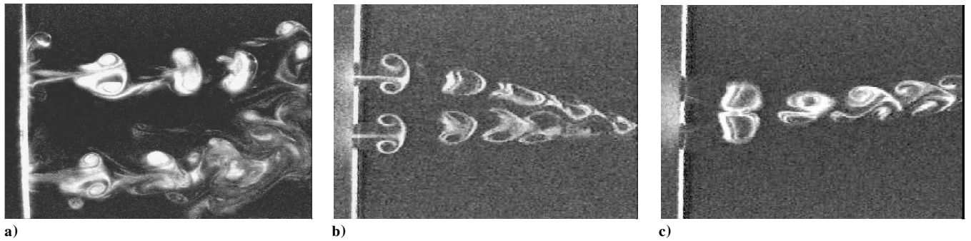
Fig. 1 Interaction between two adjacent synthetic jets in quiescent conditions. Spacing between orifices varies: a) 20, b) 8, and c) 6 mm; excitation frequency is 50 Hz, exit velocity 5 \text{ m s}^{-1} , and diameter of orifices 3.5 mm in all cases.
